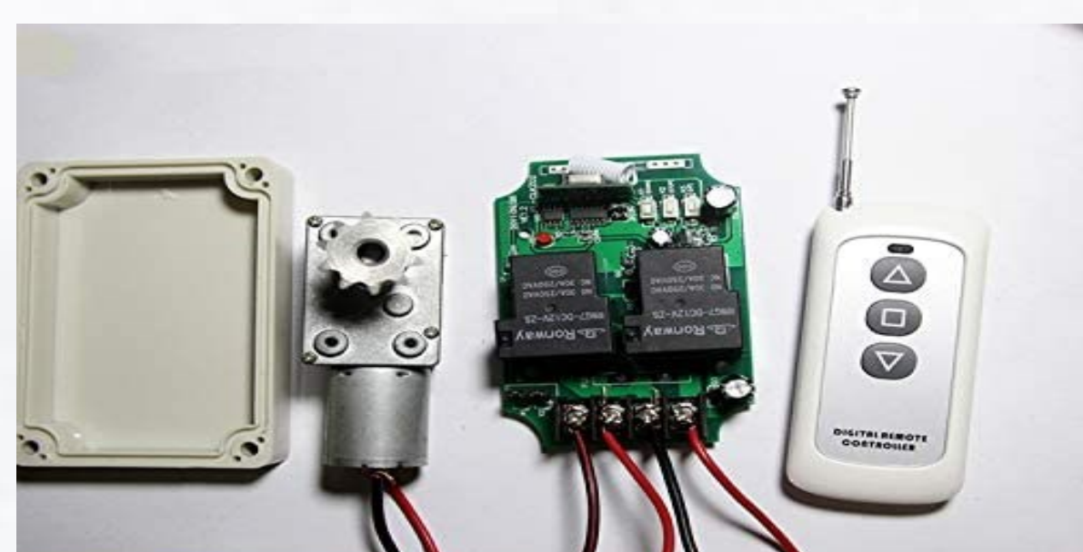
DC Motor to control a door
